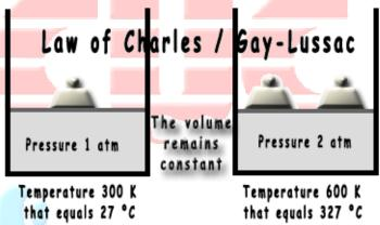
When the tanks are filled up, they heat up because the gas is compressed, so if they are filled to 200 bar, when cooled, they will have a lower pressure. We should not be surprised therefore if when checking the pressure, it gives us a reading lower than 200 bar; it is normal, even if the tanks were filled to 200 bar initially.
